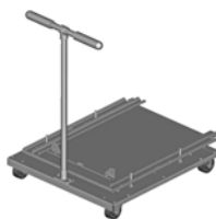
Roll-out Design (Frame 8 shown) A roll-out cart is required for Frames 8...10 drives and Frame 9...10 option bay chassis. The roll-out cart has an adjustable curb height of 0...182 mm (0...7.2 in.) and curb offset/reach of 0...114 mm (0...4.5 in.). See page 200 for information to order the roll-out cart.
