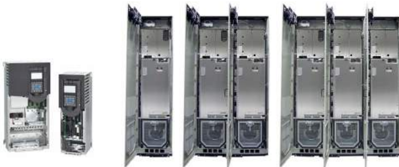
Wall Mount Frames 1...7 IP00/IP20, NEMA/UL Type Open Drive Includes a DC link choke on all Frames and internal brake transistor, standard on Frames 1...5, and optional on Frames 6 and 7.
